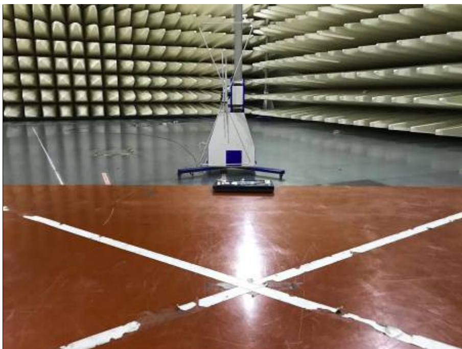
Radiated Emissions Test Setup (30-1000MHz)
