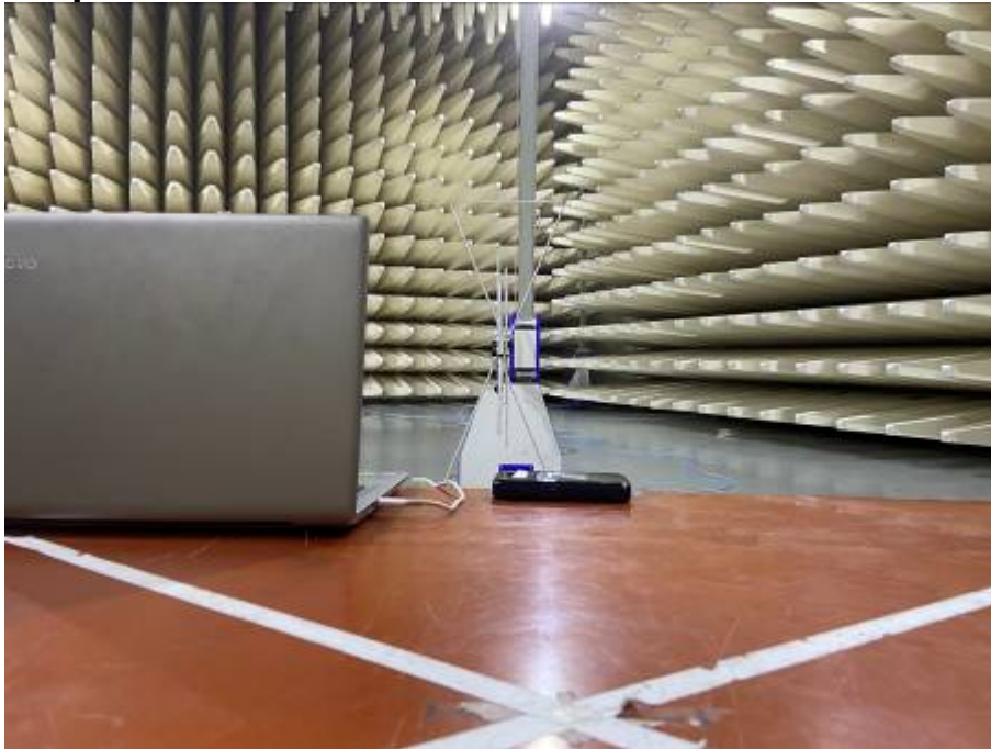
Radiated Emissions Test Setup (with laptop) (30-1000MHz)
