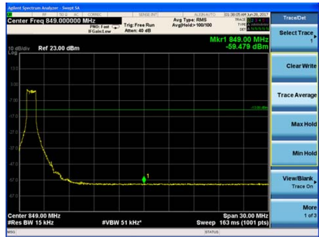
LTE Band 26 16QAM 1.4MHz CH-High 1RB
