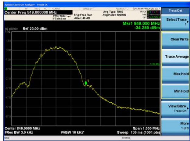
LTE Band 5 QPSK 1.4MHz CH-High 1RB
