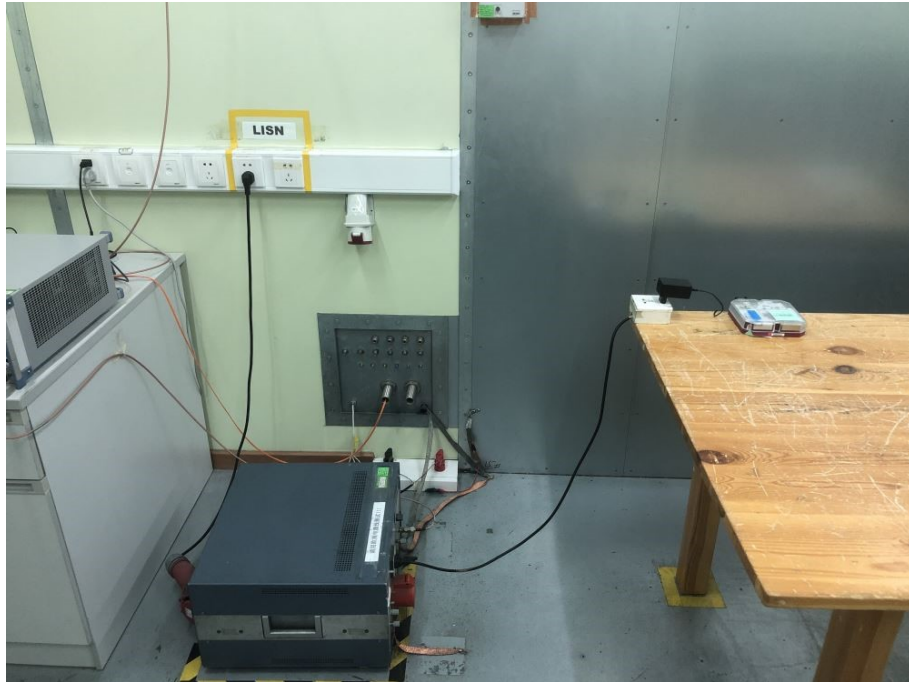
Photograph 3: Set-up for Conducted Emission on AC mains
