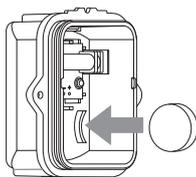
3. Check the RTR-500A1/A2 rubber packing for abrasions, cuts and dirt. If the packing is in good condition, insert into the grooves making sure that it is properly fit.
