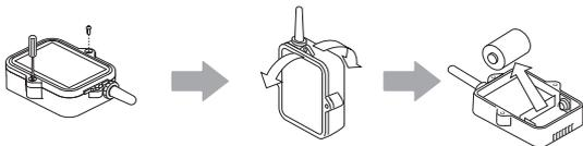
2. Attach the double-sided adhesive tape to the back of the drying agent and fix to the inner side of the RTR-500A1/A2.
