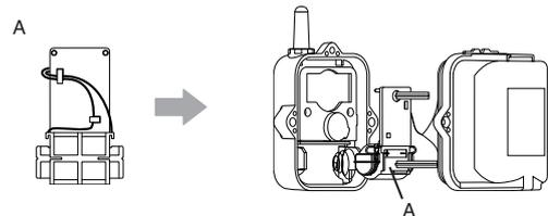
**Caution:** If the electrical wires are not properly in their grooves, the lid may not completely close. Please make sure that the wires are in their grooves before continuing.
