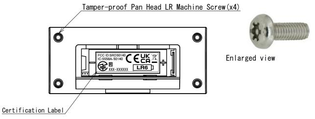
The label is placed in the battery compartment. The product is shipped without a battery installed. The user will see the label when installing the battery.
