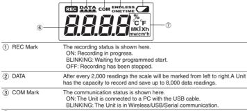
(4) Recording Mode Upon reaching capacity of 8,000 readings, the oldest data is overwritten Upon reaching capacity of 8,000 readings, recording will automatically
