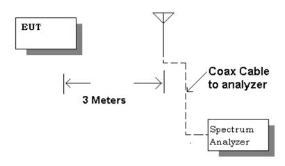
METHOD OF MEASUREMENT: The procedure used was ANSI standard C63.4-2003 & the FCC/OET Guidance on Measurements for Spread Spectrum Systems – Public Notice DA 00-705 dated March 30th, 2000.
