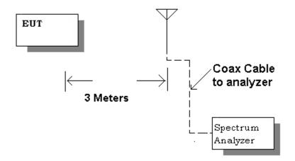
**METHOD OF MEASUREMENT:** The procedure used was ANSI standard C63.4-2003 & the FCC/OET Guidance on Measurements for Spread Spectrum Systems – Public Notice DA 00-705 dated March 30<sup>th</sup>, 2000.
