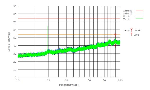
Note: A spectrum @1960MHz is downlink signal from RF tester. This is used to set EUT in idle mode. This is not a spurious emission from EUT.
