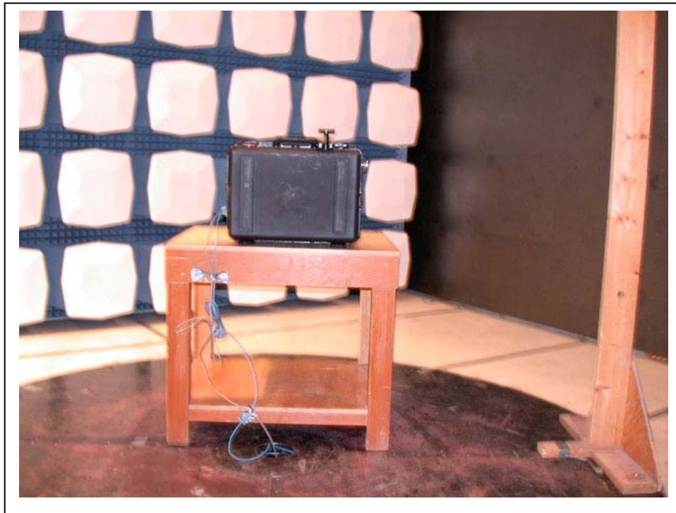
Picture of Radiated Emissions test setup:
