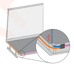
Make sure wiring does not go through any sharp or bare metal holes. Use grommets or caulk to protect wire from bare metal.
