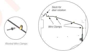
Wiring Attached to Panel
