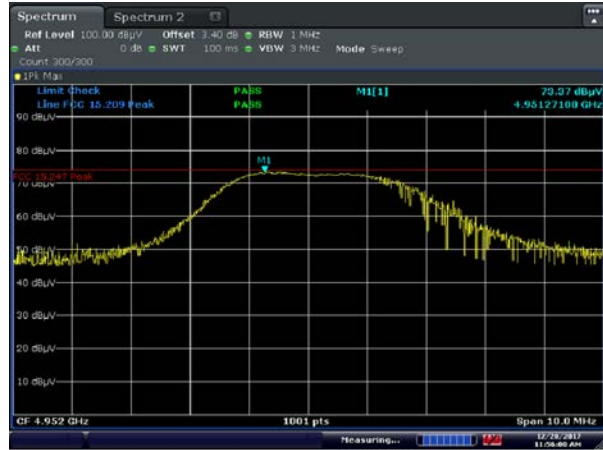
Figure 8.2-6: 2 nd harmonic emissions, High CH
