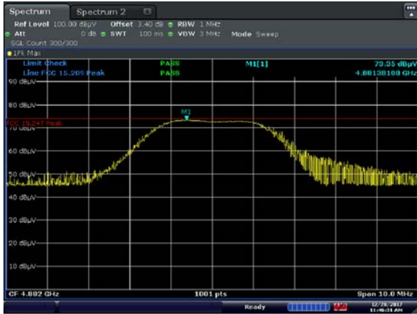
Figure 8.2-5: 2 nd harmonic emissions, Mid CH
