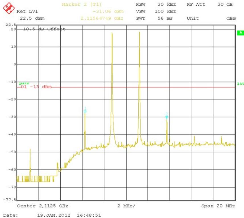
**Inter-modulation, High-band edge**
