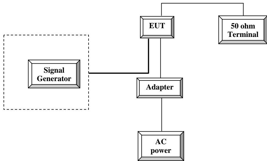
Block Diagram of Test Setup
