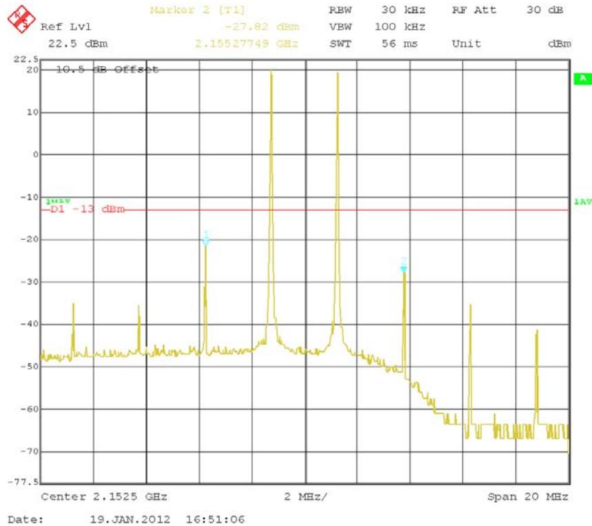
**Conducted Spurious Emission at Antenna Terminals -Low Channel**
