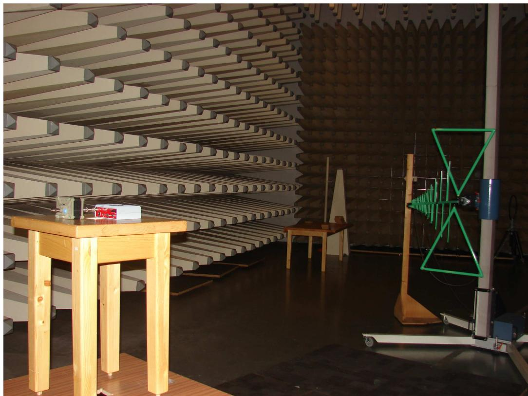
**PHOTOGRAPH 2: Test place configuration for testing radiation emission over 1 GHz**
