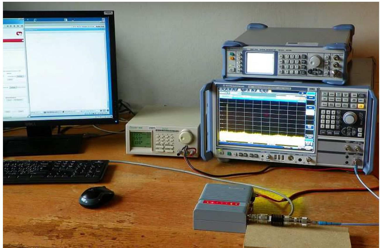
PHOTOGRAPH 4: Test site for conducted emissions (Test set up)
