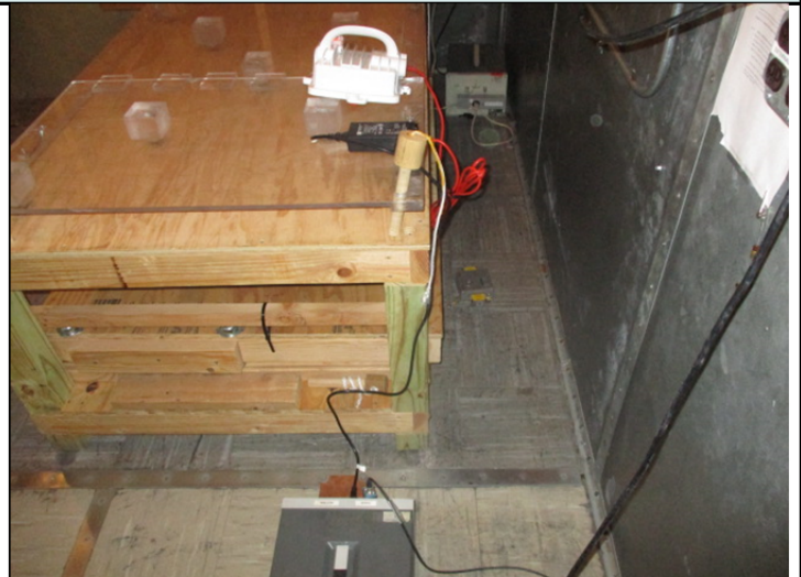
Conducted Emissions EUT Setup Side View
