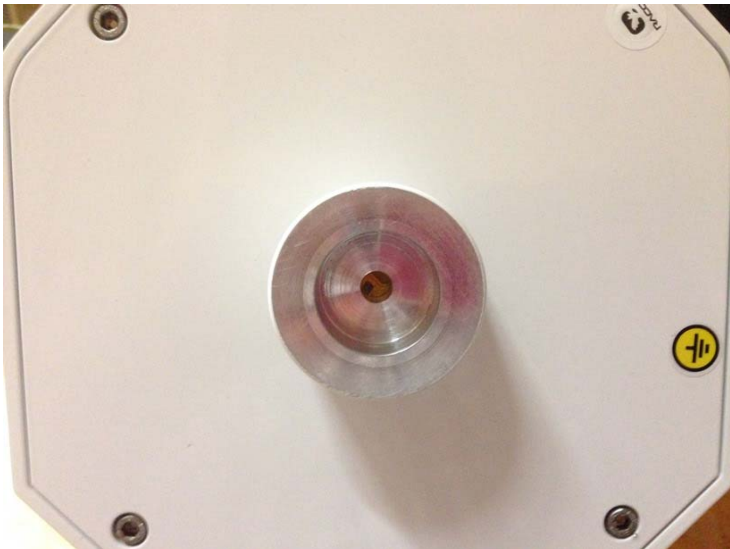
Side 2 of 6, Detail of Waveguide Port
