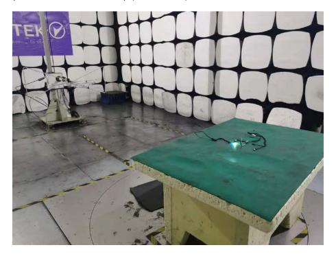
Spurious Emission Test Setup (Above 1GHz)
