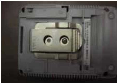
Fixing of belt fixture
