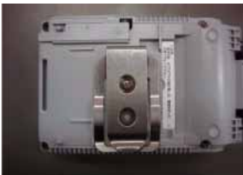
Fixing of belt fixture
