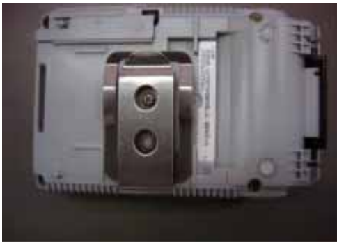
Fixing of belt fixture
