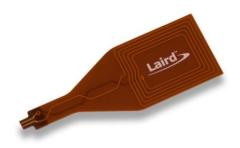
This NFC flex PCB antenna is included with the DVK-BL6xx products. It was tested with the BL65xx series of modules for NFC applications and use.
