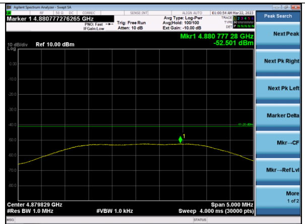
Ch 18 Spurious Emission – 4880.8 MHz
