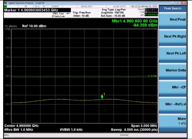
Ch 26 Spurious Emission – 4960.6 MHz
