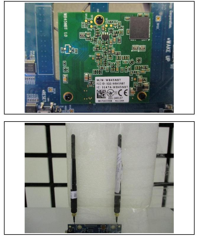
**Radiated Emission Above 1GHz Test**
