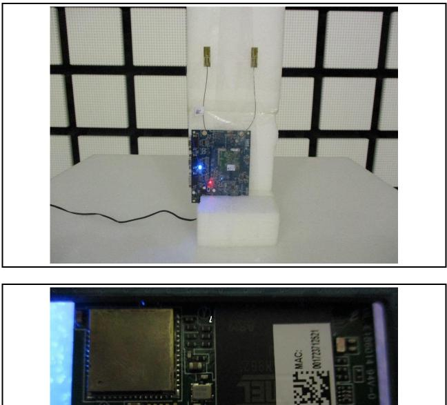
**Radiated Emission Above 1GHz Test**
