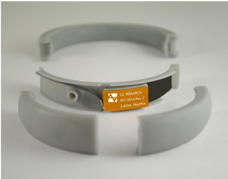
Figure 28: FlexPIFA integrated into bracelet
