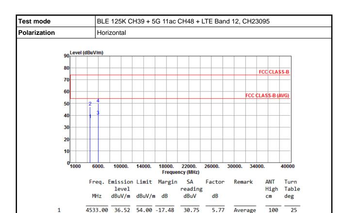
Note 1: Emission Level (dBuV/m) = SA Reading (dBuV/m) + Factor\* (dB)
