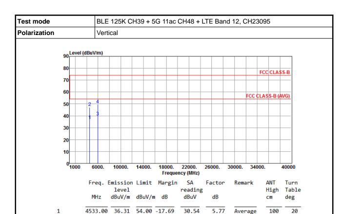
Note 1: Emission Level (dBuV/m) = SA Reading (dBuV/m) + Factor\* (dB) \*Factor includes antenna factor , cable loss and amplifier gain
