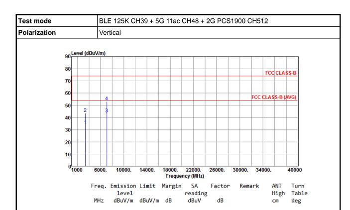
Note 2: Margin (dB) = Emission level (dBuV/m) – Limit (dBuV/m).
