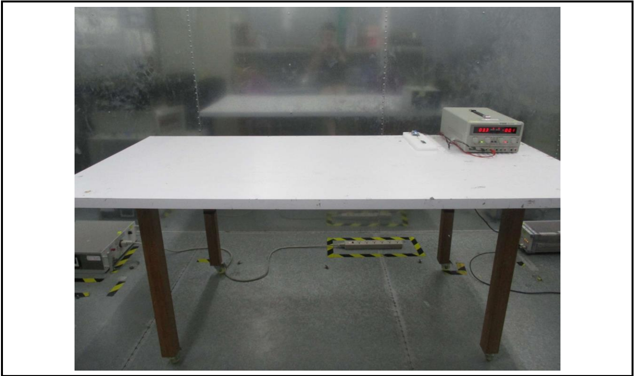
Conducted Emission Test (For Antenna 3_NanoBlade-IP04)
