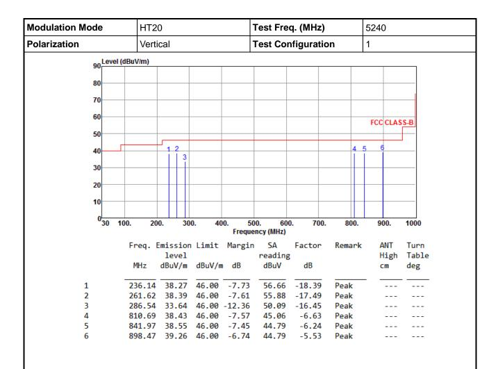
\*Factor includes antenna factor, cable loss and amplifier gain
