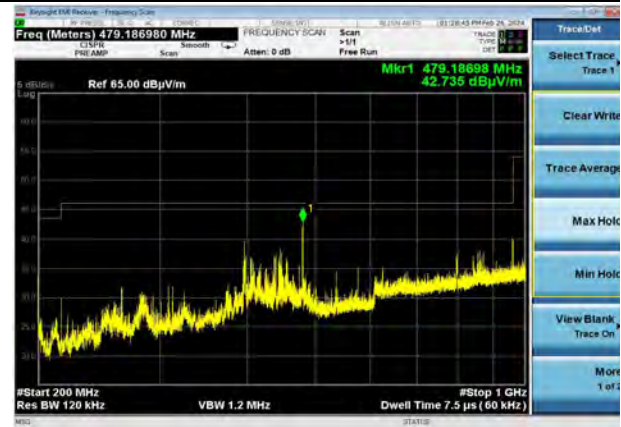
802.11b | Channel 6 | 1 Mbps | 200-1000 MHz | Vertical
