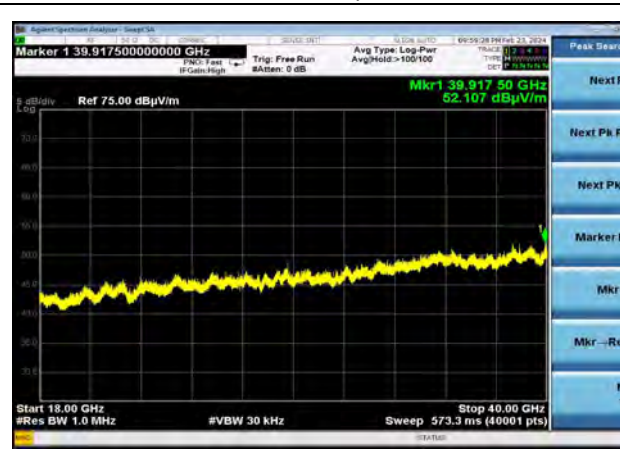
802.11b | Channel 6 | 1 Mbps 18000-40000 MHz | Vertical
