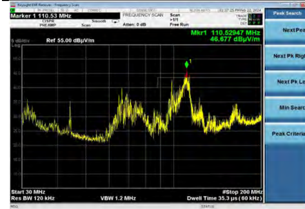
802.11b | Channel 6 | 1 Mbps | 30-200 MHz | Vertical
