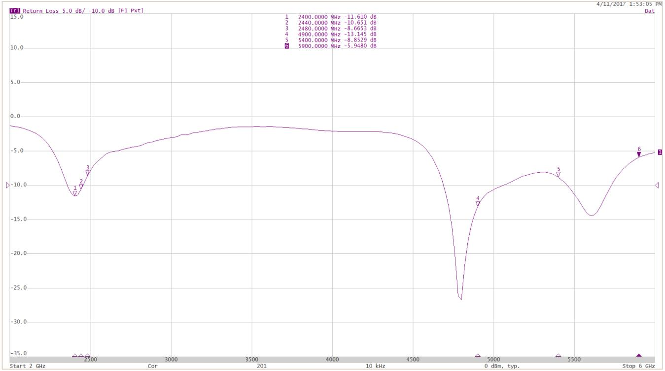
Figure 2: Antenna RL measured on a 1.5 mm-thick plate of polycarbonate
