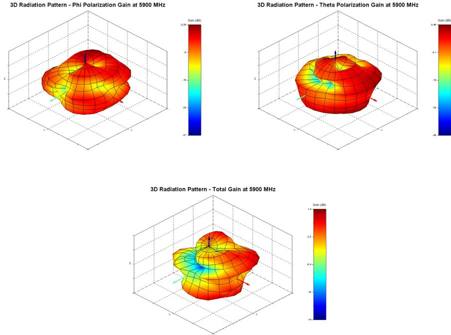
Figure 20: Phi, Theta, and total gain plots
