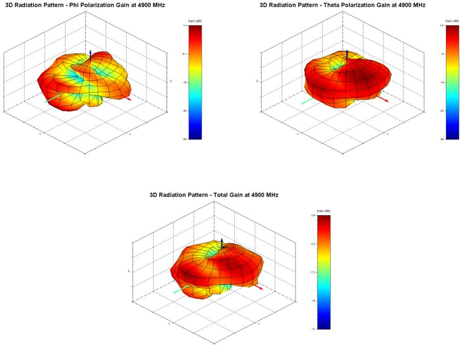
Figure 25: Phi, Theta, and total gain plots
