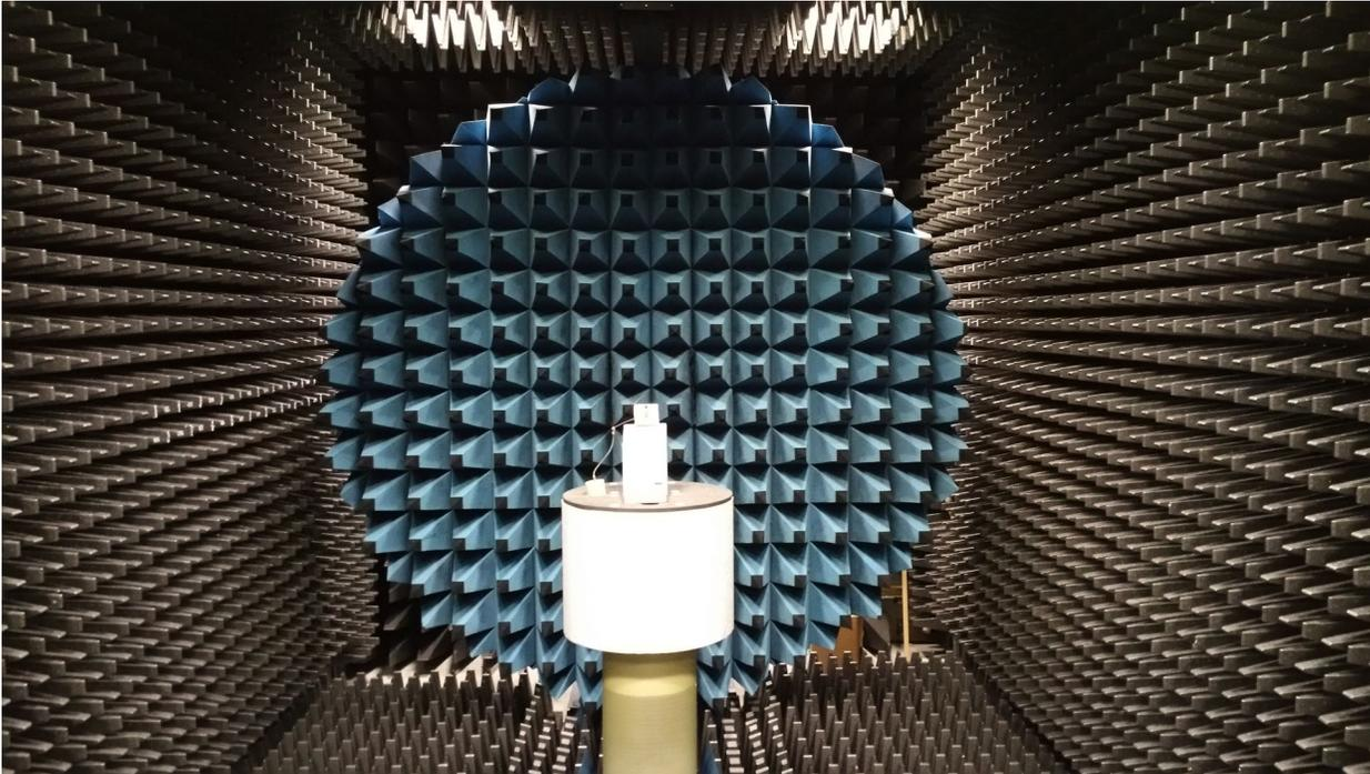
*Figure 1: Antenna chamber*
