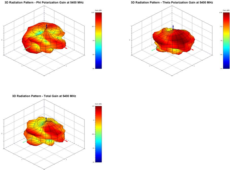
Figure 27: Phi, Theta, and total gain plots
