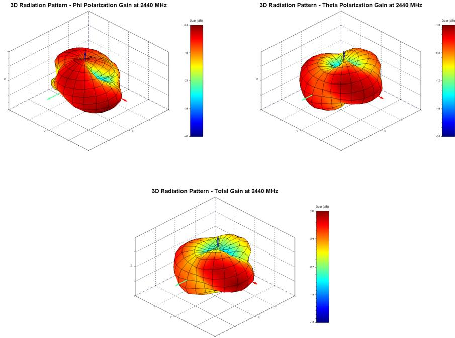
Figure 23: Phi, Theta, and total gain plots
