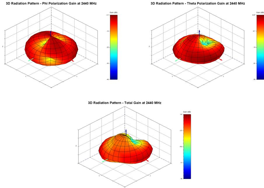
Figure 14: Phi, Theta, and total gain plots
