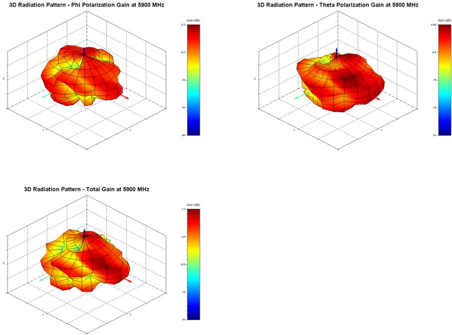
Figure 29: Phi, Theta, and total gain plots
