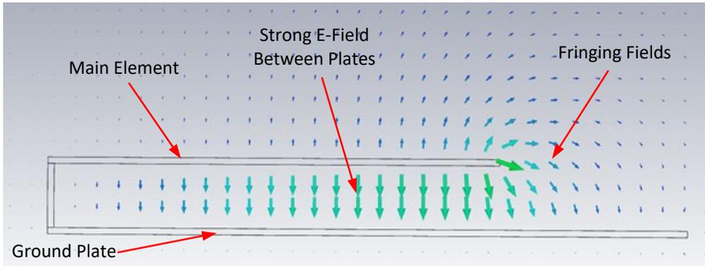
Figure 30: E-field radiation from FlexPIFA – taken from CST simulation
