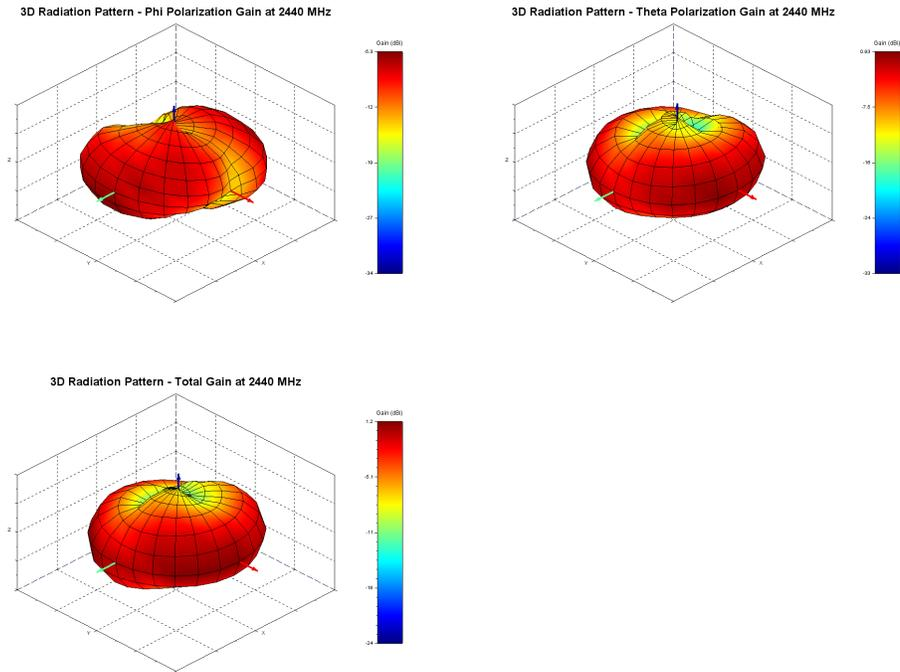
Figure 5: Phi, Theta, and total gain plots
