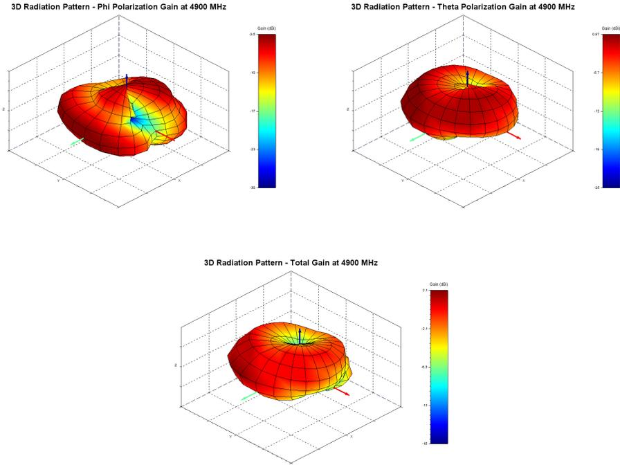
Figure 7: Phi, Theta, and total gain plots
