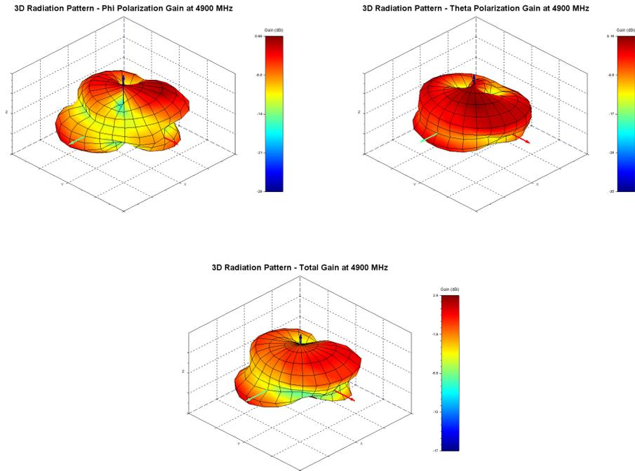
Figure 16: Phi, Theta, and total gain plots
