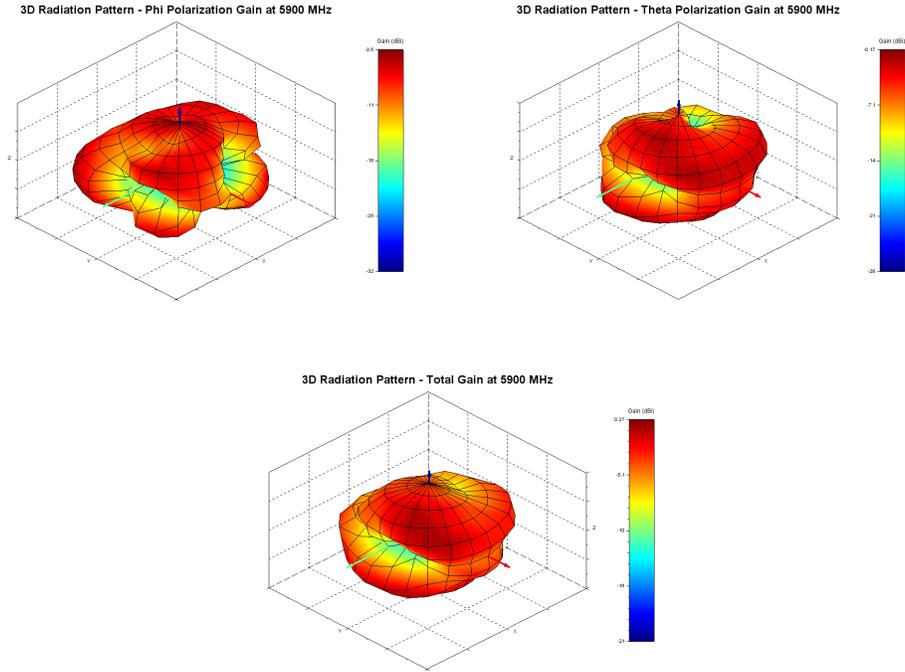
Figure 11: Phi, Theta, and total gain plots
