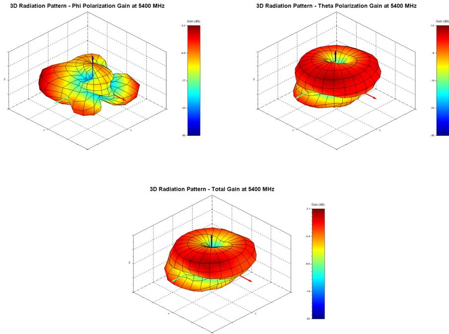
Figure 9: Phi, Theta, and total gain plots
