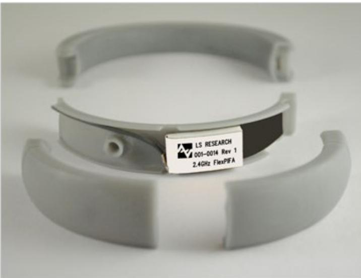
**Figure 39: FlexPIFA integrated into bracelet**
