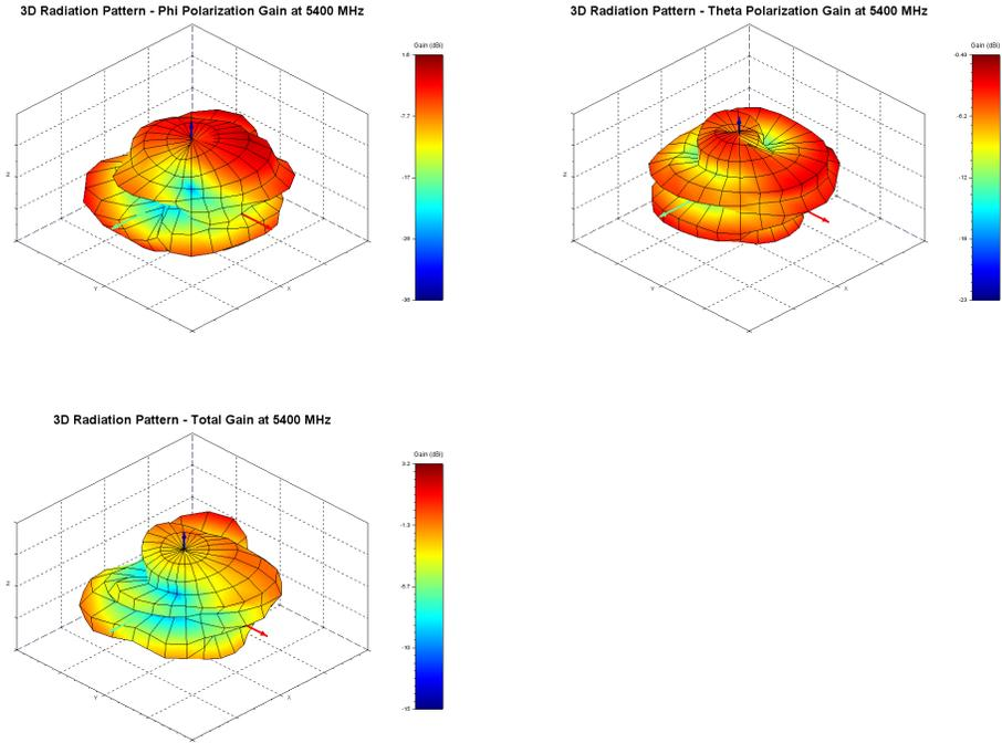
Figure 18: Phi, Theta, and total gain plots
