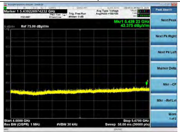
802.11a | Channel 144 | 6 Mbps | Y Plane 4000-5470 MHz | Horizontal
