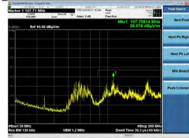
802.11a | Channel 165 | 6 Mbps | Y Plane 30-200 MHz | Horizontal
