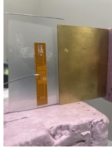
Figure 14: Return Loss measured on a 2.1 mm-thick sheet of polycarbonate with varying parallel edge ground distances
