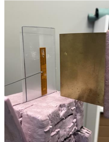
Figure 16: Return Loss measured on a 2.1 mm-thick sheet of polycarbonate with varying ground distances
