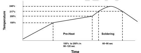
Figure 16: Recommended Reflow Profile
