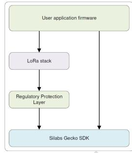
Figure 8: Firmware block diagram - native C development
