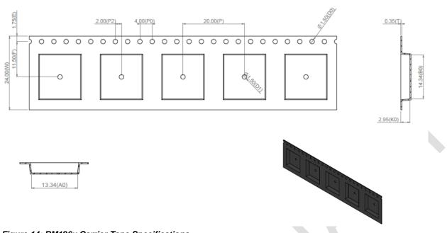
Figure 14: RM126x Carrier Tape Specifications
