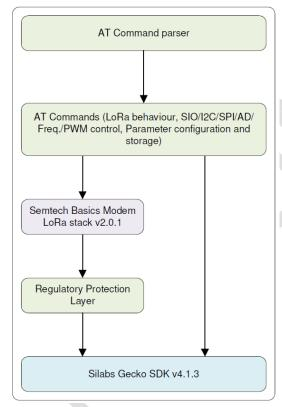
Figure 7: Firmware block diagram - AT firmware
