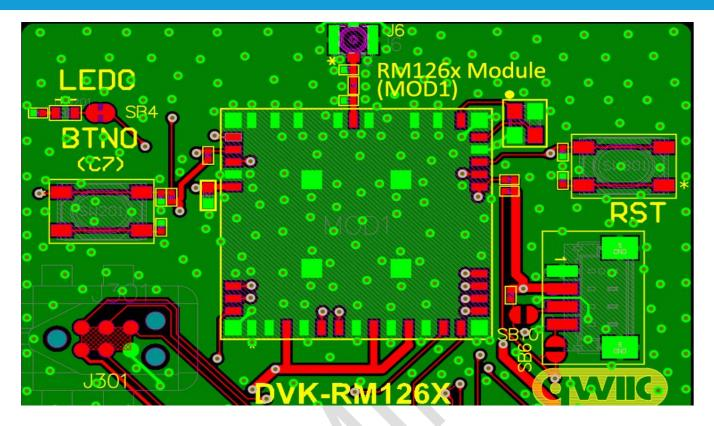
Figure 11: RM126x module PCB placement and grounding (shown in green) on DVK-RM126x PCB (part of DVK-RM126x PCB with RM126x module shown only) with RM126x module placed near the edge.
