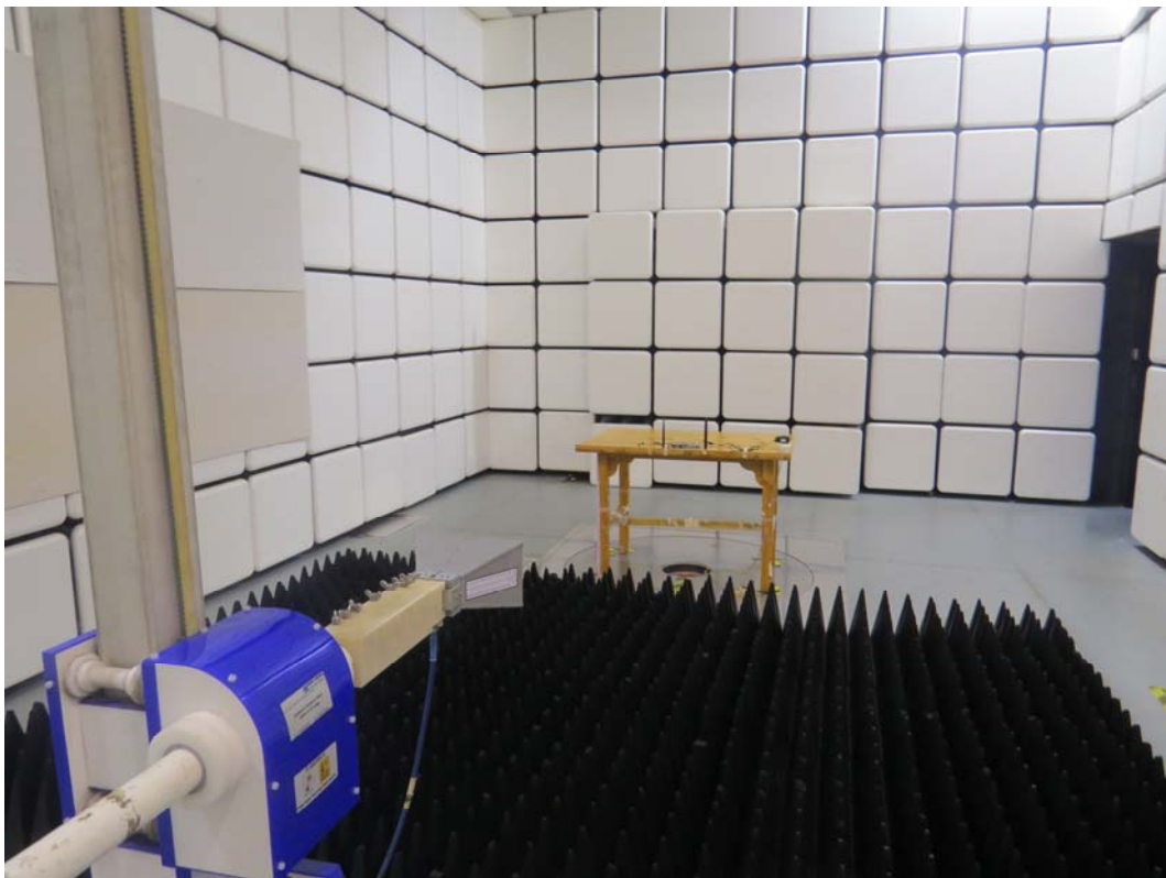
Picture 2: Radiated Spurious Emissions Test setup
