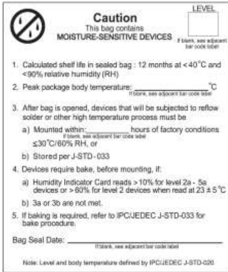
Figure 8: Sona MT320 M.2 1420 Moisture Sensitivity Level Label
