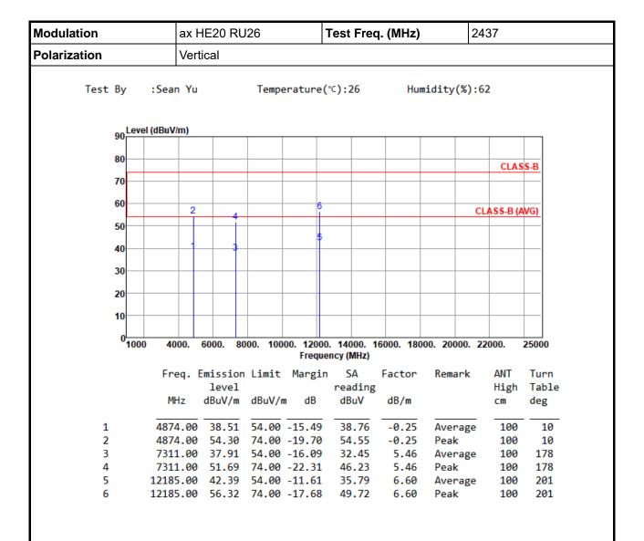
Note 1: Emission Level (dBuV/m) = SA Reading (dBuV) + Factor\* (dB/m) \*Factor includes antenna factor, cable loss and amplifier gain
