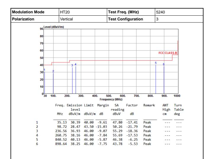
Note 1: Level (dBuV/m) = Read Level (dBuV/m) + Antenna Factor (dB) + Cable Loss (dB) - Preamp Factor (dB). 2: Over Limit (dBuV/m) = Limit Line (dBuV/m) - Level (dBuV/m).
