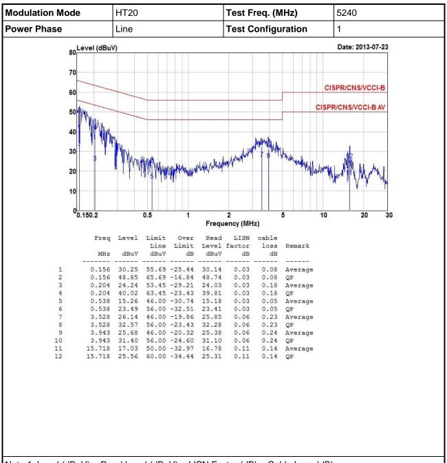
Note 1: Level (dBuV) = Read Level (dBuV) + LISN Factor (dB) + Cable Loss (dB).
