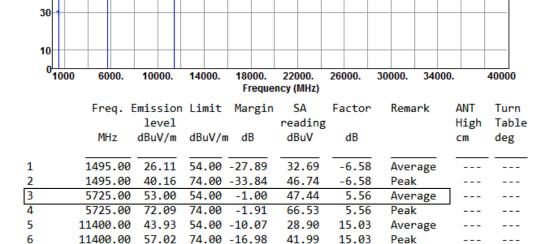
Note 1: ">20dB" means spurious emission levels that exceed the level of 20 dB below the applicable limit. Note 2: For restricted bands, the peak measurement is fully sufficient, as the max field strength as measured with the Peak-Detector meets the AV-Limit so that the AV level does not need to be reported in addition.
