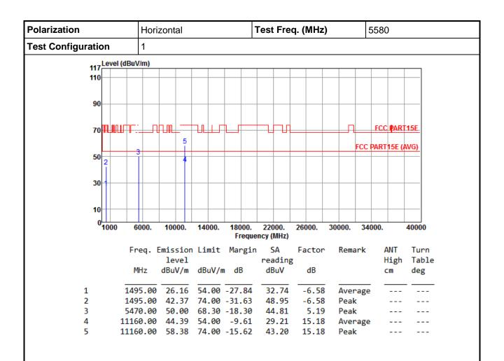
Note 1: ">20dB" means spurious emission levels that exceed the level of 20 dB below the applicable limit. Note 2: For restricted bands, the peak measurement is fully sufficient, as the max field strength as measured with the Peak-Detector meets the AV-Limit so that the AV level does not need to be reported in addition.
