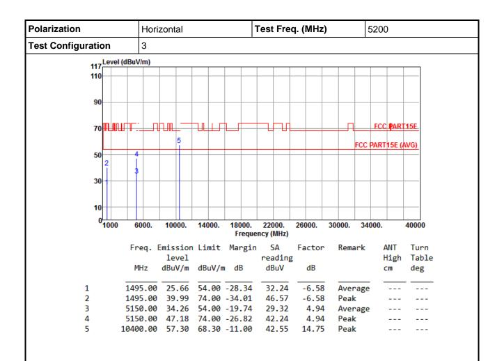
Note 1: ">20dB" means spurious emission levels that exceed the level of 20 dB below the applicable limit.
