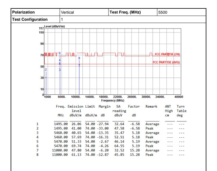
Note 1: ">20dB" means spurious emission levels that exceed the level of 20 dB below the applicable limit. Note 2: For restricted bands, the peak measurement is fully sufficient, as the max field strength as measured with the Peak-Detector meets the AV-Limit so that the AV level does not need to be reported in addition.
