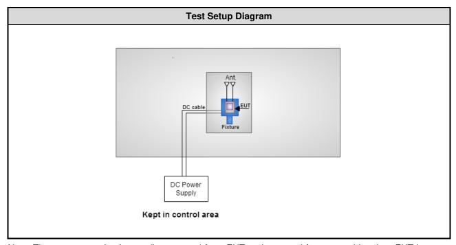
Note: The support notebook was disconnected from EUT and removed from test table when EUT is set to transmit continuously.
