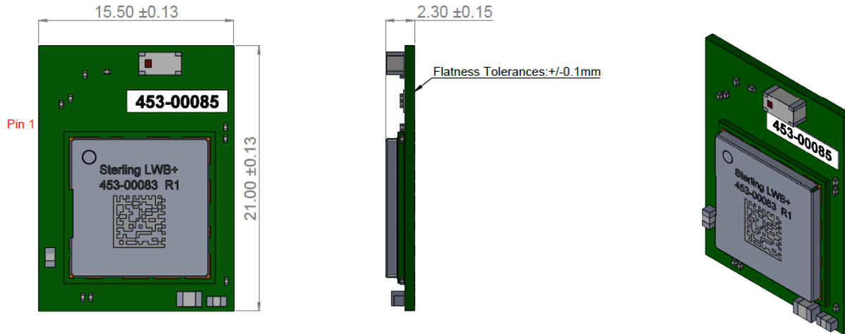
Figure 18: Sterling LWB+ MHF® 4 and chip antenna module dimension
