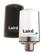
Laird's unique patented Phantom® antenna is ideal for cell, GSM, PCE, WIFI, 802.11 and Bluetooth wireless applications. Measuring only 2.7" tall, the Phantom 800 MHz to 5.8 GHz antenna models' revolutionary design features a robust IP67 rated mechanical solution with frequency agility, low visibility, wide bandwidth and a low angle radiation pattern that is superior to traditional gain antennas in most applications, both outdoor and indoor.
