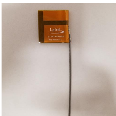
Figure 20: Recommended cable routing
