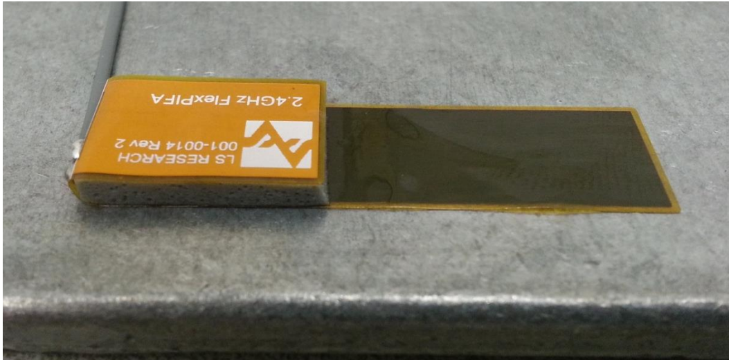
Figure 24: FlexPIFA mounted on metal
