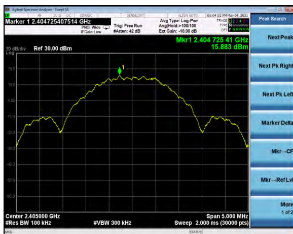
Neg4dBm, channel 11, reference plot 15.9 dBm
