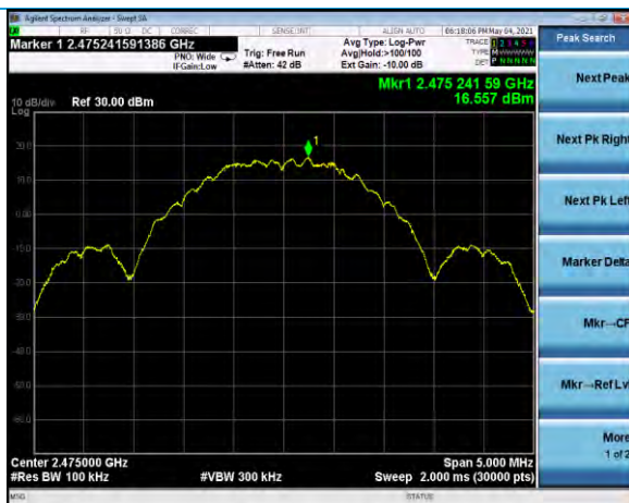
Neg4dBm, channel 25, reference plot 16.6 dBm
