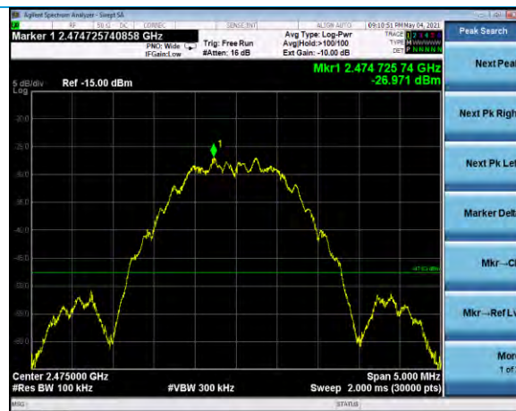
Neg40dBm, channel 25, reference plot -27.0 dBm
