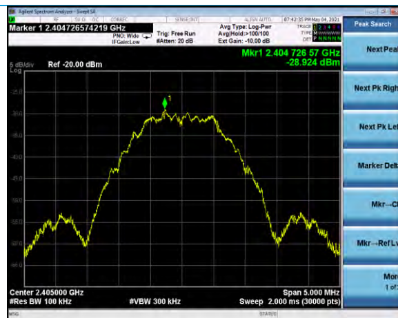
Neg40dBm, channel 11, reference plot -28.9 dBm
