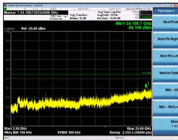
Conducted TX Spurious 2.5-25 GHz Channel 19, neg40dBm
