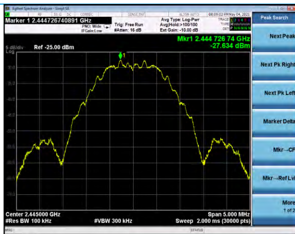
Neg40dBm, channel 19, reference plot -27.6 dBm
