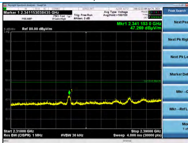
2.31-2.39 GHz, Horizontal Antenna Vertical EUT, Channel 11
