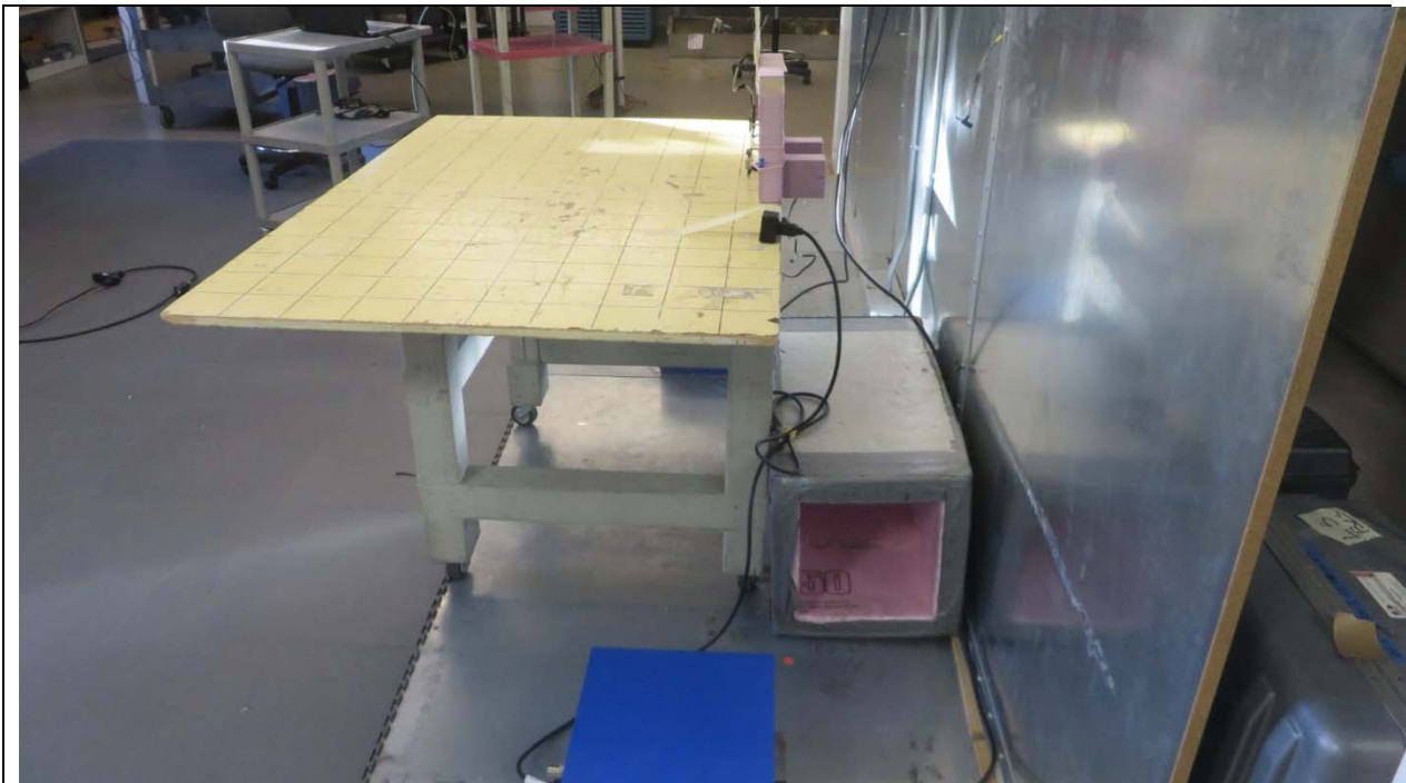
Description: AC Mains Conducted Emissions
