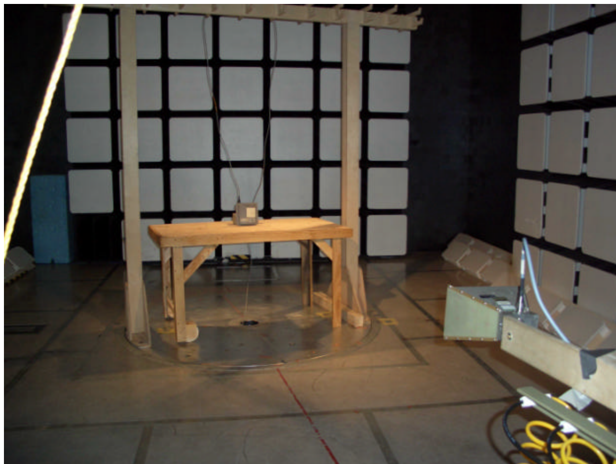
Figure 7-1: WLAN 6220 Corporate Service Unit Radiated Emissions Set-up
