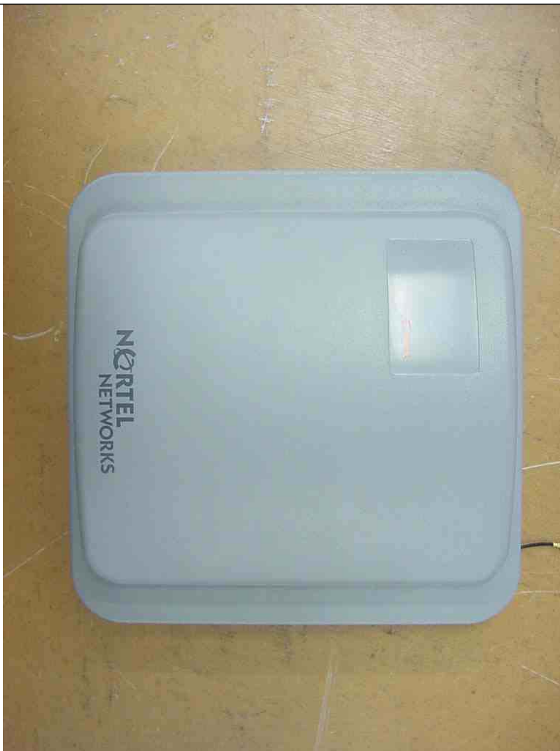
Enclosure with 5 GHz Antenna
