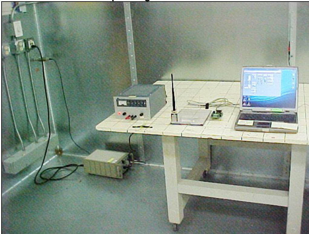
View of the EUT setup during the Conducted Emissions Test
