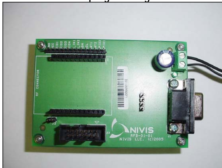
Top view of the RS-232 programming and interface fixture.
