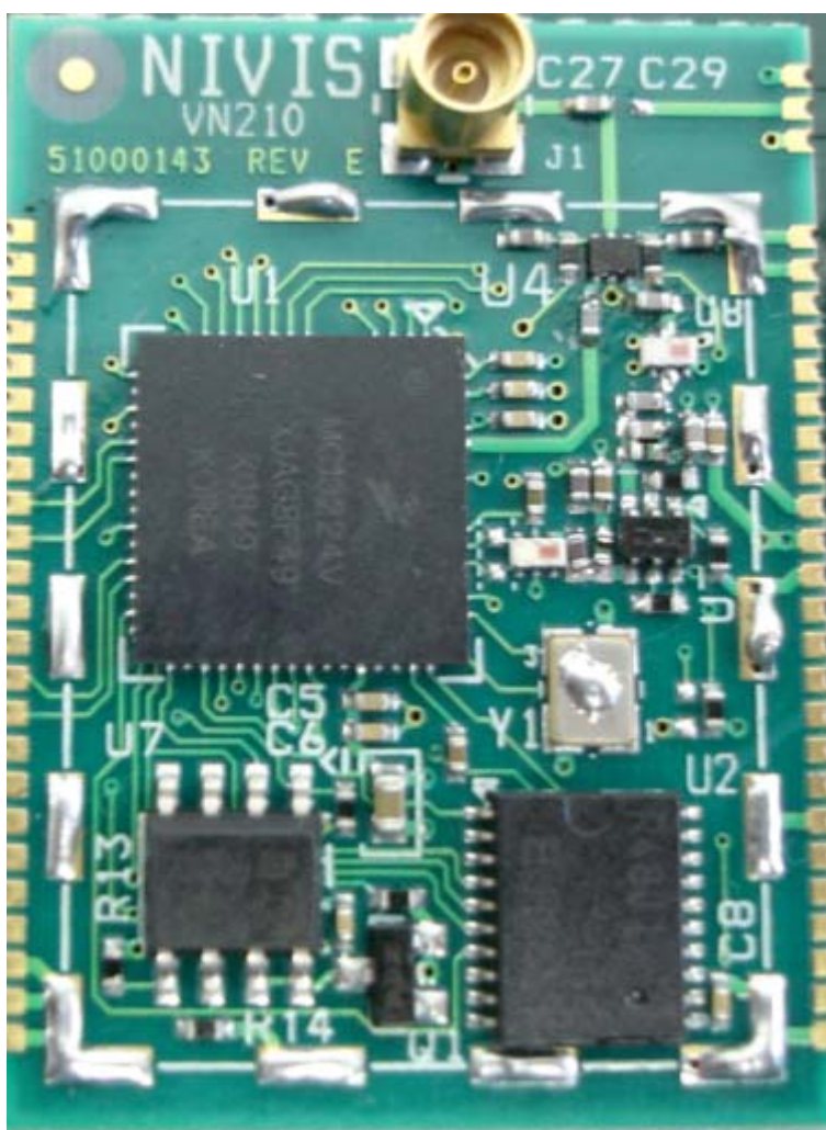
Internal Photograph 1. Top of Transmitter Module, Shield Removed
