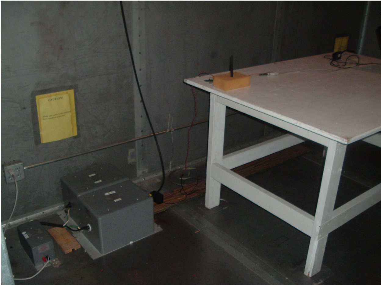
Figure 5 - Conducted Emissions Measurement Setup
