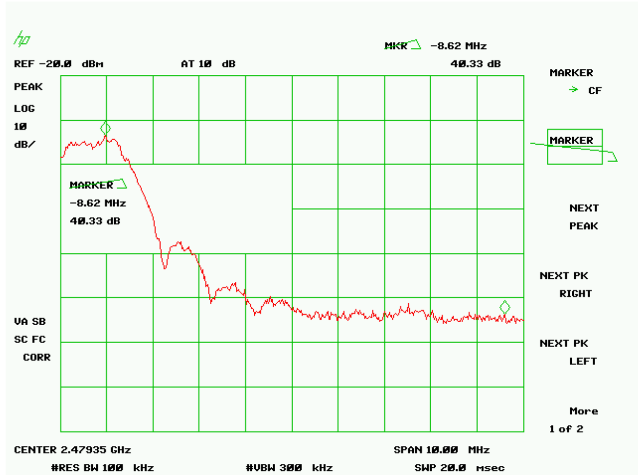
Figure 23 - Band Edge Compliance - High Channel Delta – Radiated – Integral Antenna
