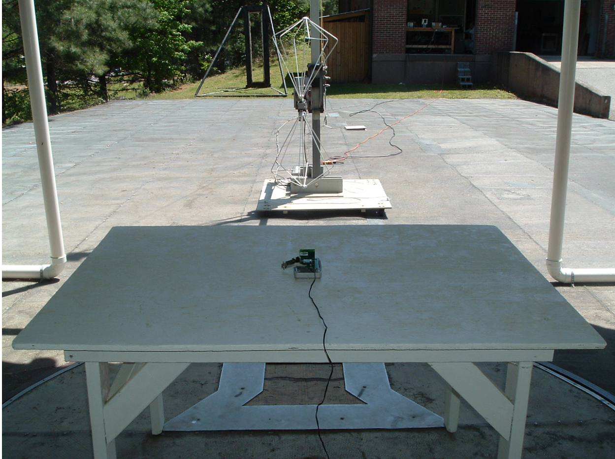
Figure 5 - Digital Radiated Emissions Measurement Setup (Rear View)
