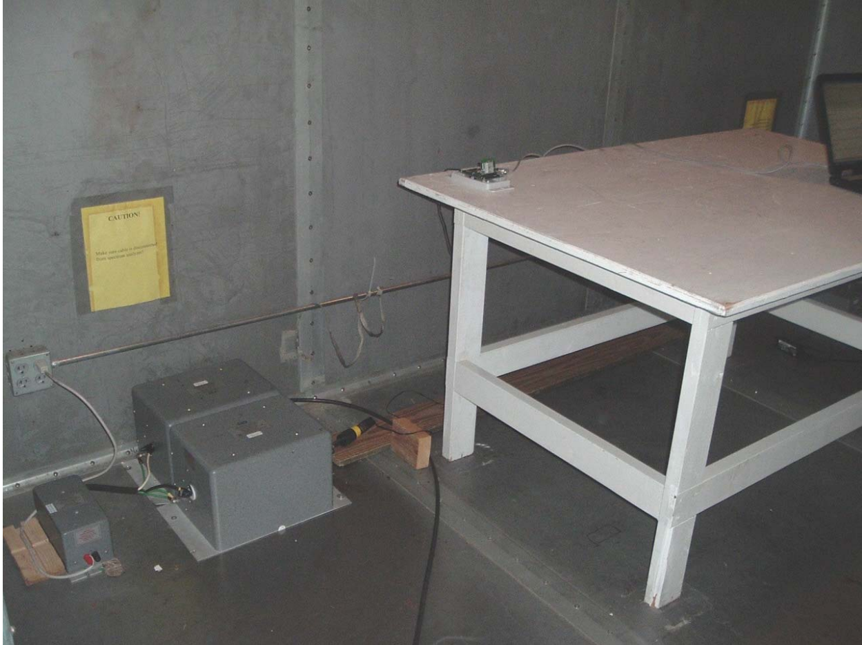
Figure 9 - Conducted Emissions Measurement Setup
