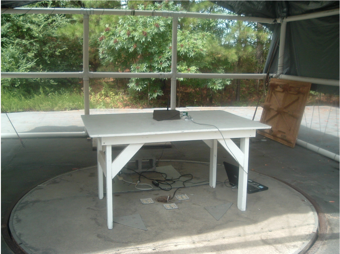
Figure 1: Radiated Test Configuration Antenna 1 Omni Antenna 5.5dBi Gain (Front View)
